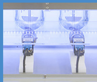
24/7 testing with LED light bar and six ethernet cameras.
