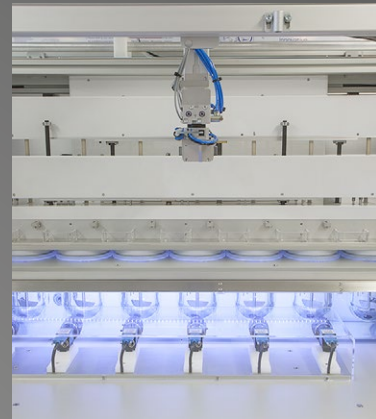
LED light strip for 24/7 video recording
